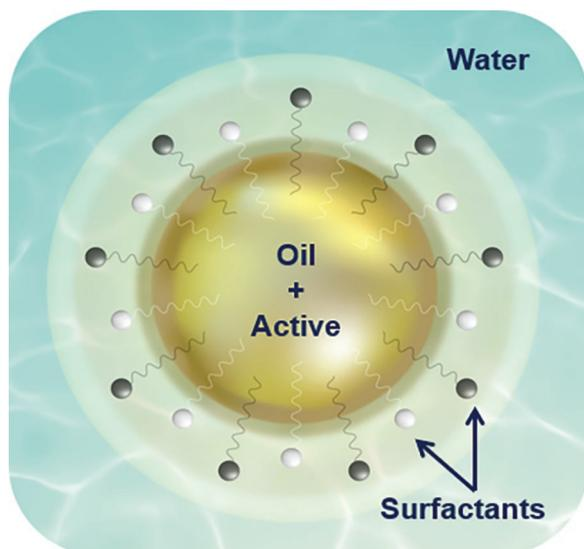
A multimolecular layer of organized surfactant, oil and water forms a robust three-dimensional bicontinuous structure around the oil droplet. PAD formulations are manufactured with low levels of surfactant in the water and oil phases, in contrast to conventional emulsions that require a large excess of surfactant in the water phase to maintain physical stability.<sup>12</sup>
